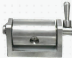
A fixed device for thick test fabric (maximum thickness of 8mm)
